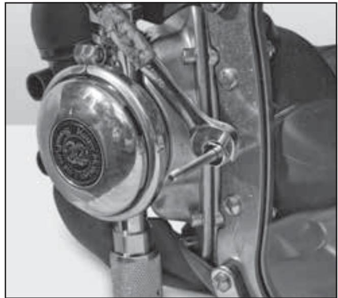
*Do not tighten the nose block packing too much or the nose block device will not slide easily.*
