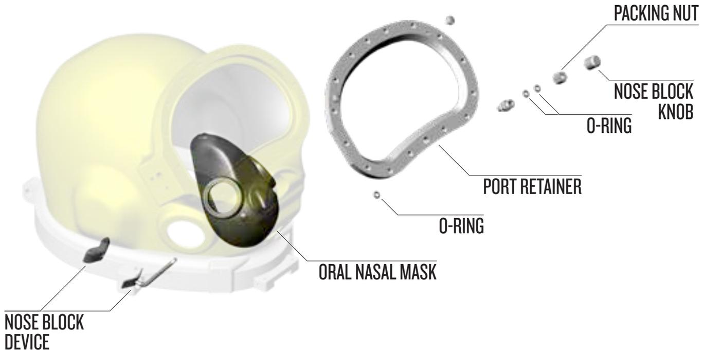
Blowapart of the nose block device and supporting hardware. (Same as found on KMB BandMasks).
