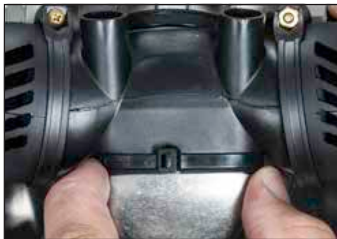
The Quad Valve must be properly connected to the regulator and the quad exhaust extension on the pod.
