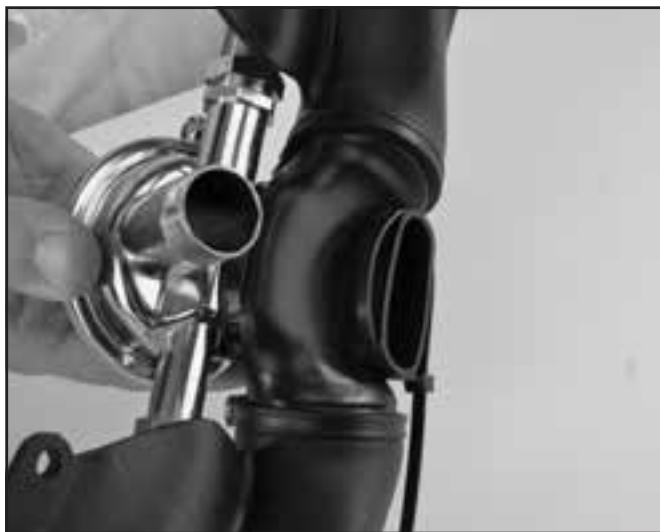
Pre-install the tie wrap.
