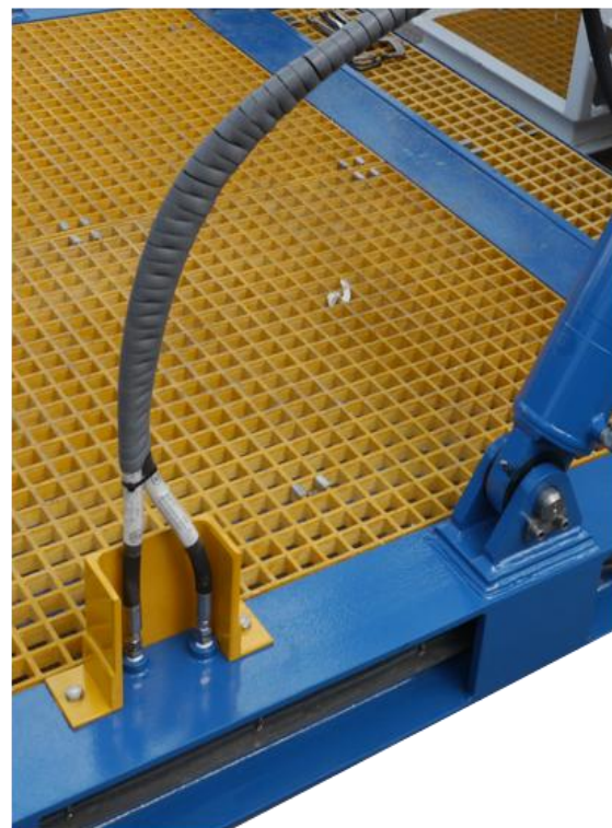
Above: Cylinder clevis & hydraulics
