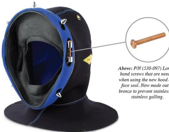
Above: P/N (530-097) Longer band screws that are needed when using the new hood and face seal. Now made out of bronze to prevent stainless on stainless galling.
