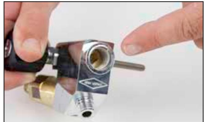
*The seat should be removed for inspection.*
