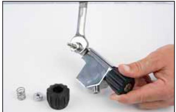
*Undo the packing nut.*
