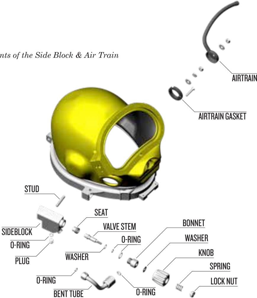
The diver controls the flow of gas through the defogger system with the control knob. The gas enters the helmet and flows through the air train which directs the gas onto the face port to help eliminate or clear fogging that forms on the face port from the diver's warm breath. In the event water gets inside, the water needs to be evacuated. Some of the air from the airtrain will force this water out through the water dump valve.
