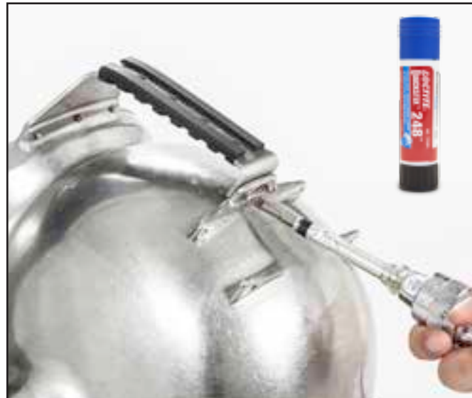
Tighten the screws on the rear of the handle see “Torque Specs” on page APNDX-19 for correct torque.
