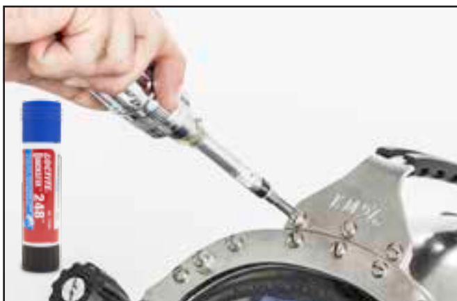
Tighten the screws on the front of the handle see “Torque Specs” on page APNDX-19 for correct torque.
