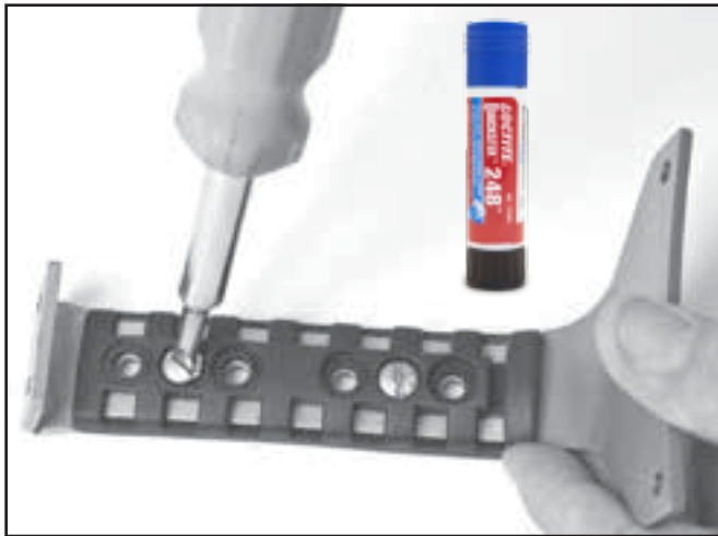
Tighten the screws to just until rubber begins to extrude. The tips will protrude slightly through the other side of the handle.
